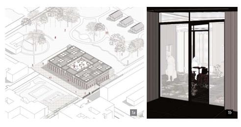
presence of green courtyards covered by sliding ETFE cushions that would work as bioclimatic greenhouses.
